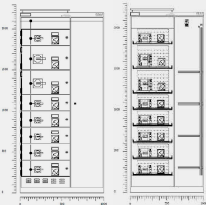
Outgoing feeder panel in modular design Plug-in technology up to 630 A
