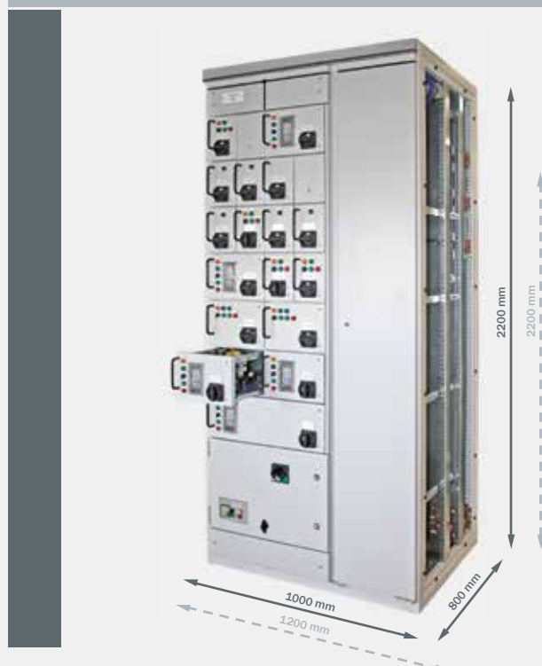
F51 panel: MCC outgoing feeder panel with 6 shuttle levels (10 x 1/4 and 6 x 1/2 slide-in units), 1 x E1H, 1 x KE400
